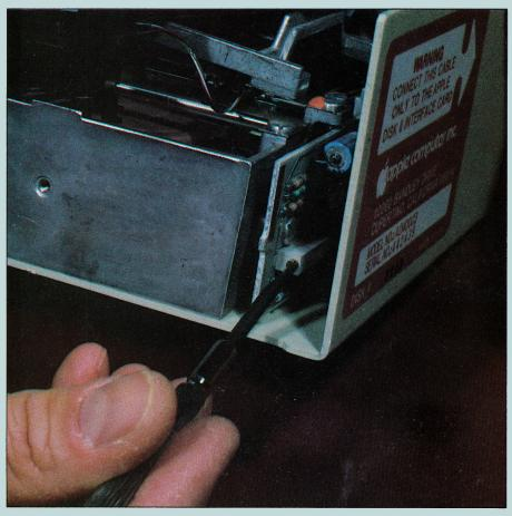
Photo 1. Locating the disk speed trimmer pot.
